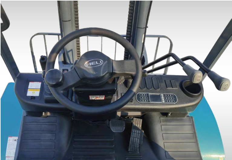
The layout of the instrument panel conforms to human-machine operating habits, integrated handle switches, integrated electro-hydraulic reversing handle, ratcheting hand brake, and more comfortable operation.
